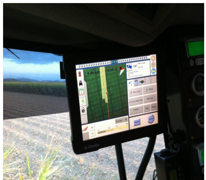
Typical Auto-Steer/Precision Ag screen installed in close to 200 machines in the Herbert
