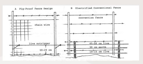
Pig-proof fences (A) are expensive to construct but are very effective. Electrifying a conventional fence (B) greatly improves its effectiveness and will add years to its life. In moist soil conditions a single live wire as in "A" will suffice.
