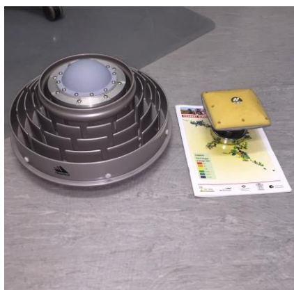
New technology Multi Constellation Choke Ring GPS Antenna on the left compared to old unit
