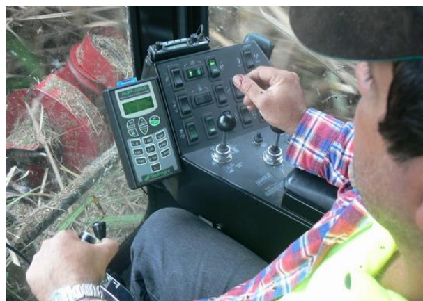
On board computer of the automatic base-cutter system
