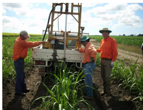
Installation of enviro-scan for monitoring soil moisture status in the drought treatment. A Chinese scientist (Dr Liao) assisting BSES researchers for field experimentation.
